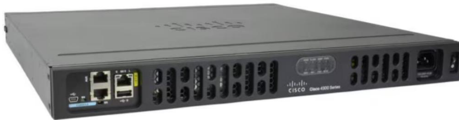
Figura 18. Router CISCO 4300 Series
